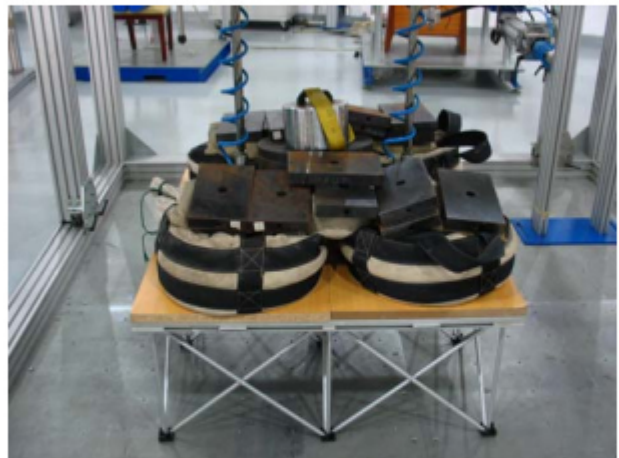
Photo 6 Bearing strength test - uniform load 1900 kg
