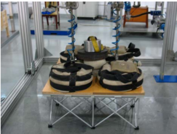
Photo 5 Bearing strength test - uniform load 1700 kg
