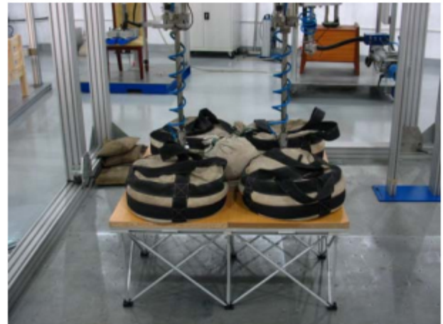
Photo 4 Bearing strength test - uniform load 1500 kg
