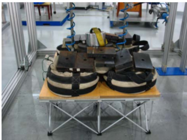
Photo7 Bearing strength test - uniform load 2000 kg
