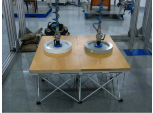
Photo 2 Bearing strength test - uniform load 500 kg
